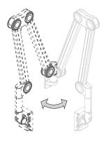
Move the arm from side to side to verify if the arm moves correctly.
